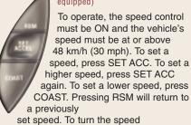
again. To set a lower speed, press COAST. Pressing RSM will return to set speed. To turn the speed
